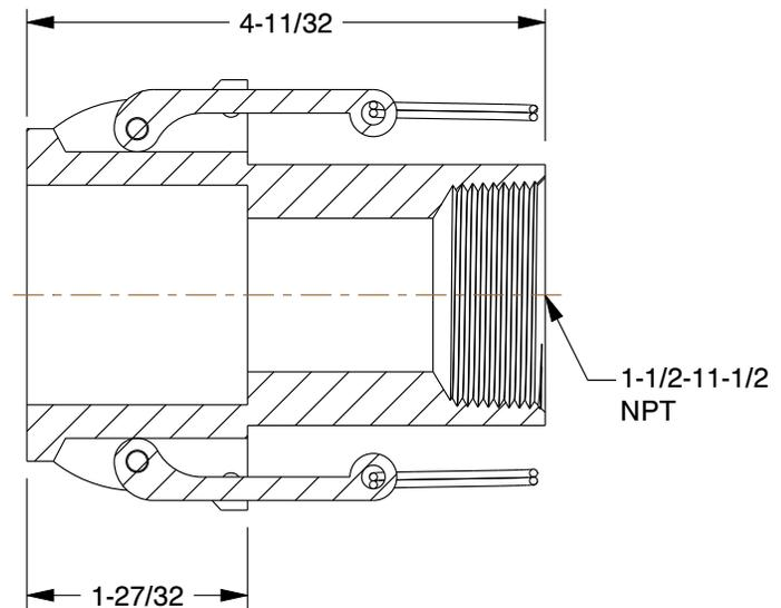
**COMPONENT** Polypropylene Cam and Groove Fittings
