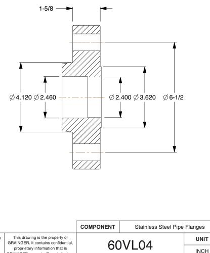
Pipe Flange: Socket Weld Flange, 316/316L Stainless Steel, 2 in Pipe Size, Class 1500 SHEET
