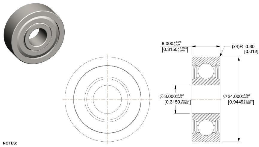
1. MATERIAL: Steel 2. ABEC TOLERANCE: 1 3. TYPE: Double Shielded 4. LUBRICATION: Dry Powder 5. ITEM: Radial Ball Bearing 6. TEMP. RANGE: 390° Fto 660°F
