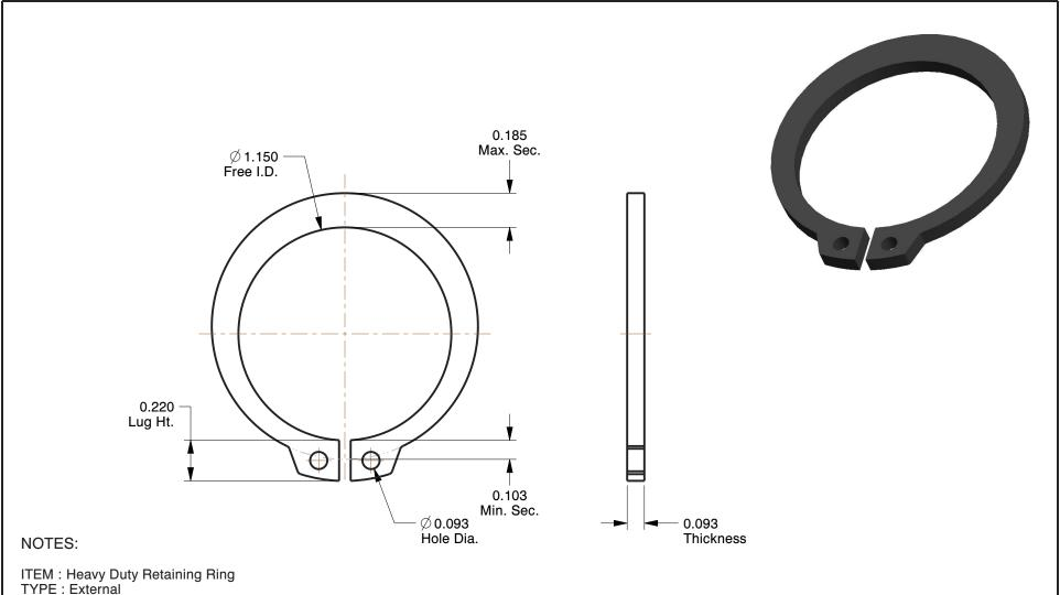
MATERIAL: Carbon Steel FINISH: Black Phosphate FOR SHAFT DIA: 1-1/4" PACKAGE QUANTITY: 10
