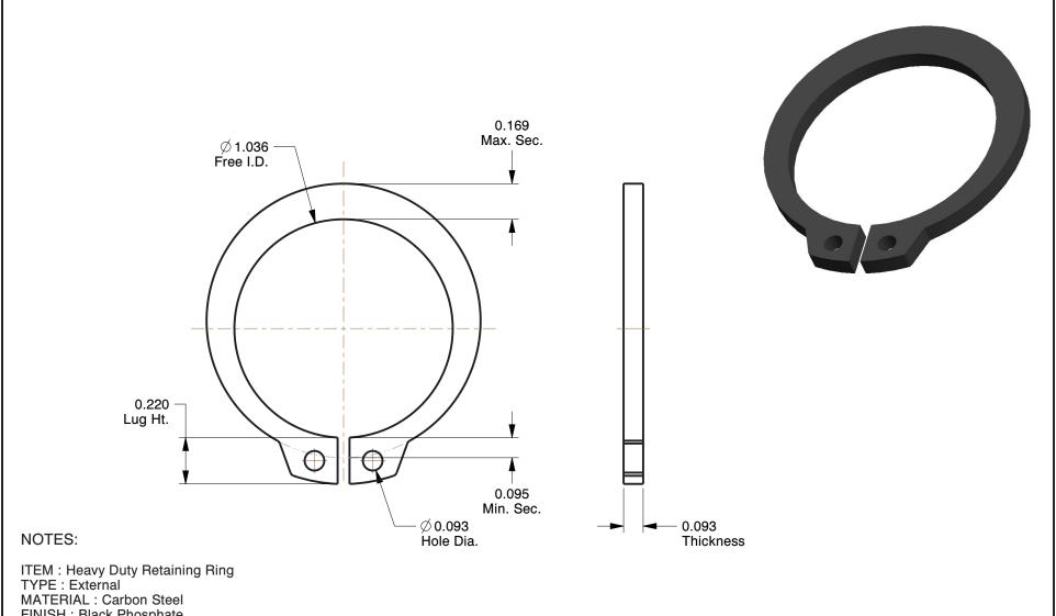
MATERIAL: Carbon Steel FINISH: Black Phosphate FOR SHAFT DIA: 1-1/8" PACKAGE QUANTITY: 10
