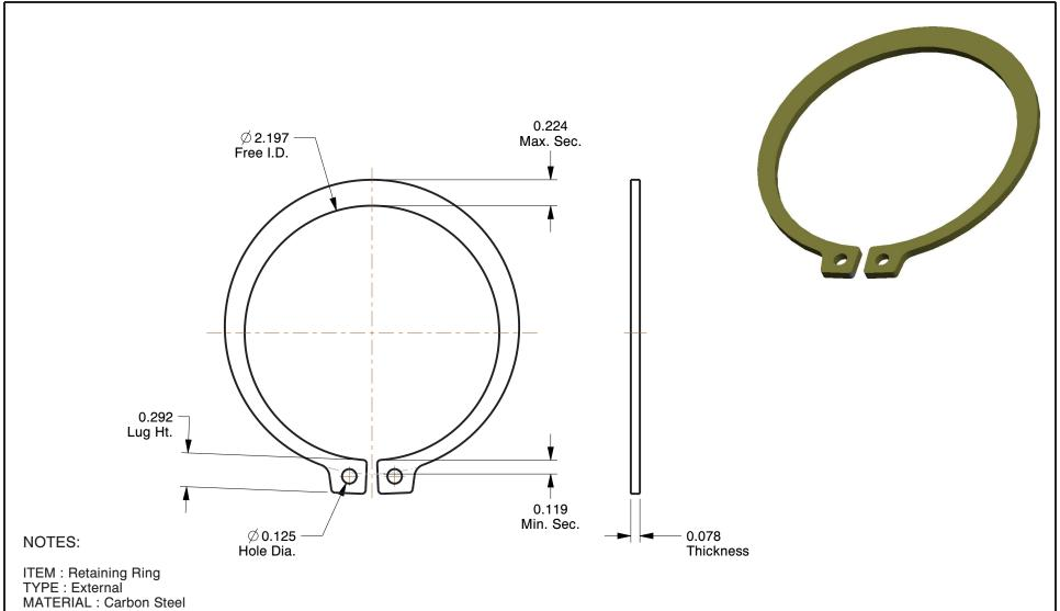
MATERIAL: Carbon Steel FINISH: Yellow Zinc FOR SHAFT DIA: 2-3/8" PACKAGE QUANTITY: 10
