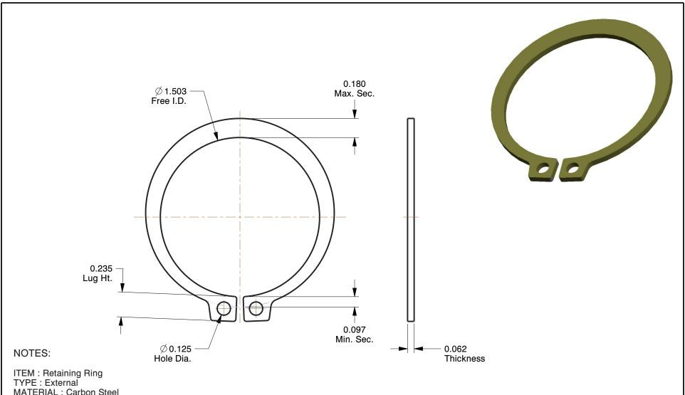
MATERIAL: Carbon Steel FINISH: Yellow Zinc FOR SHAFT DIA: 1-5/8" PACKAGE QUANTITY: 25
