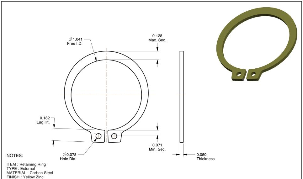
MATERIAL: Carbon Steel FINISH: Yellow Zinc FOR SHAFT DIA: 1-1/8" PACKAGE QUANTITY: 25
