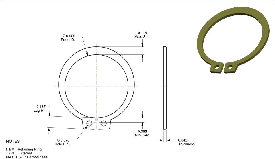
MATERIAL: Carbon Steel FINISH: Yellow Zinc FOR SHAFT DIA: 1" PACKAGE QUANTITY: 50
