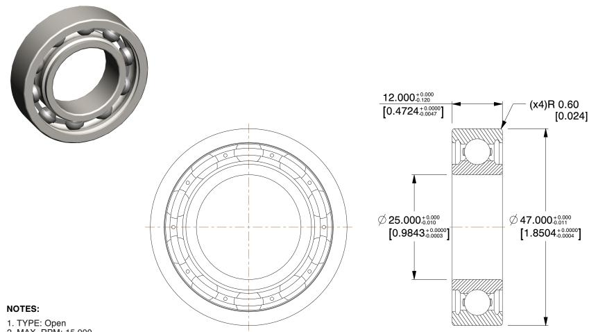
2. MAX. RPM: 15.000 3. ABEC TOLERANCE: 1 4. BEARING MATERIAL: Steel
