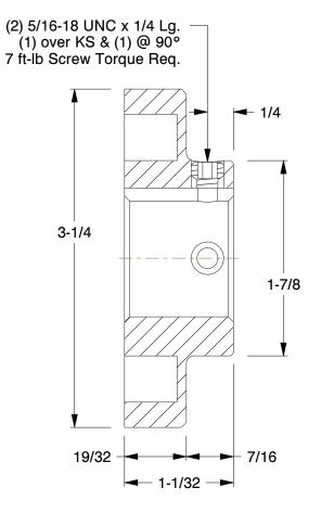
6. MATERIAL: Sintered Carbon Steel 7. MAX. ANGULAR MISALIGNMENT: 1°
