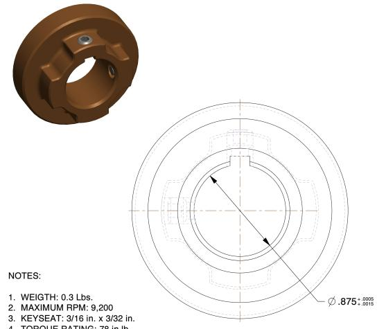
(2) 1/4-20 UNC x 1/4 Lg. (1) over KS & (1) @ 90° 3 ft-lb Screw Torque Req. **⋖** 3/16 2-1/16 1-1/2 13/32 <del>-</del> 13/32 25/32
