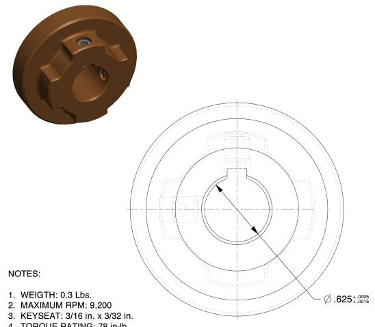
(2) 1/4-20 UNC x 3/16 Lg. (1) over KS & (1) @ 90° 3 ft-lb Screw Torque Req. **⋖** 3/16 2-1/16 1-1/2 13/32 <del>></del> 13/32 25/32
