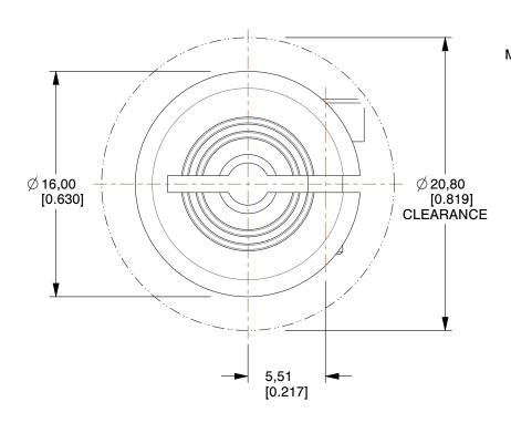
$9,00^{+0,076}_{-0,254}$  $[0.354^{+0.0030}_{-0.0100}]$ M3x8 Forged Clamp Screws 2.5 mm Hex Wrench Size 2.1 Nm Seating Torque Ø 6,00+0,05  $\left[0.236^{+0.002}_{-0.001}\right]$
