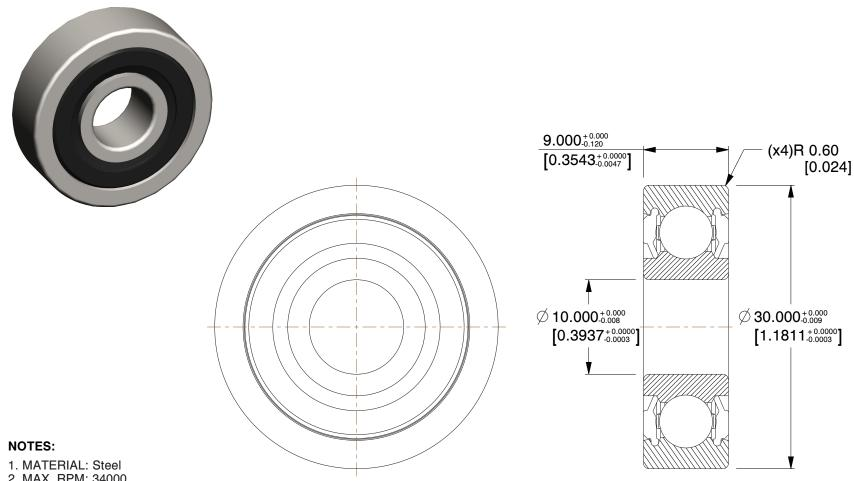
2. MAX. RPM: 34000 3. TYPE: Double Sealed
