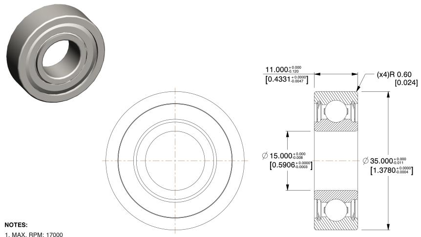
2. ABEC TOLERANCE: 1 3. LUBRICATION: Grease 4. TYPE: Double Shielded 5. ITEM: Radial Ball Bearing
