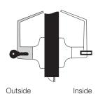
\*Lever handles are Free Wheeling in locked position. Shaded area denotes Free Wheeling lever.
