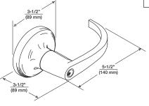
See page 10 & 11 to order interchangeable core cylinder. Dimensions are in inches (millimeters).
