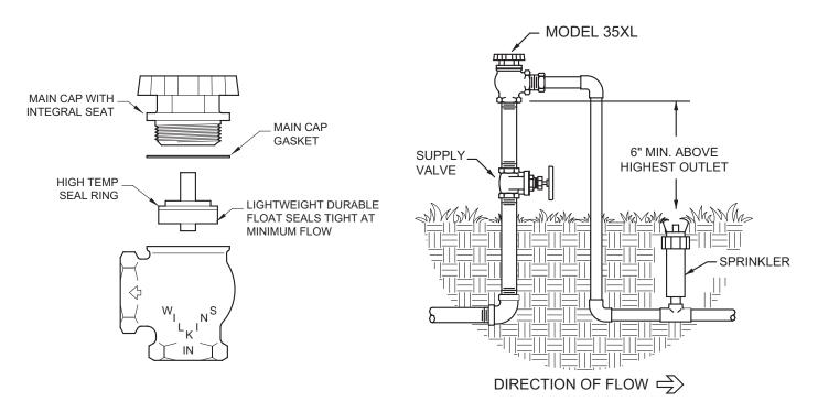
**CAUTION**: This device should never be used in installations that are under continuous pressure. Therefore, never place a shut-off or check valve downstream of AVB's.
