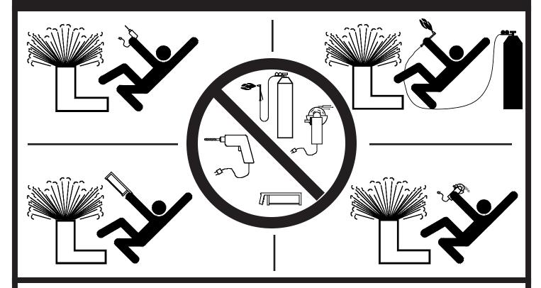
Danger of explosion. Do not drill, grind, saw, weld or use a torch on this product. Doing so could result in serious injury, death or property damage.
