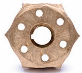
WORN DRIVE PLUG Accelerated wear due to lack of drain holes in a look-alike brush
