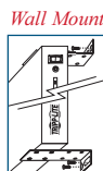
Remove, reorient and reinstall hardware along sides of outlet strip. Mount on wall.
