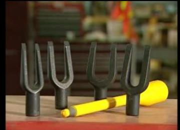
Tie Rod/Ball Joint Separators are available in four sizes •11/16" •15/16" •1 1/8"
