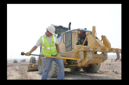
Pin Drivers are specifically designed for removing pins from heavy equipment.
