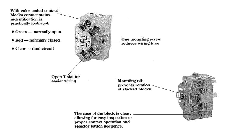
The Series J Fingersafe contact blocks no longer have a webbed wire separator, but an open T slot that accepts fork tongue and Ferrule type cable ends/connectors. These contact blocks accept a wire range of #12-24 AWG. With a control circuit rating of 10 amps 600 VAC maximum and a logic circuit rating of 5 VDC, 1 mA minimum, one standard contact block can fulfill requirements for both control and logic circuitry.
