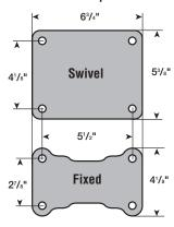
TS5/TF5 top plates have fixing holes to suit 3/8" diameter bolts.
