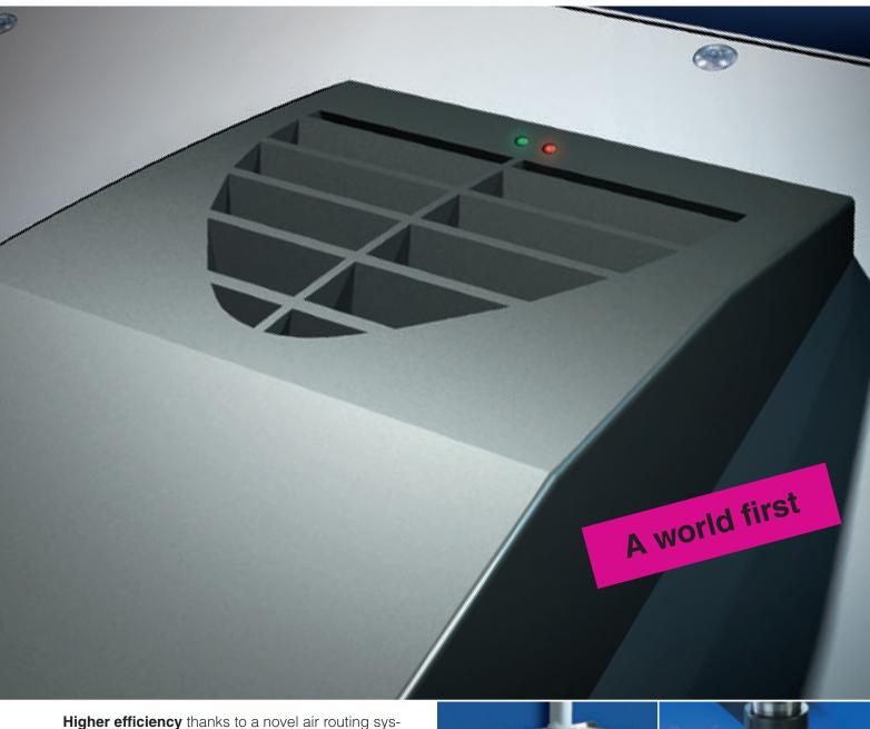
**Higher efficiency** thanks to a novel air routing system, and optimum activation of the Peltier elements and fans through pulse width modulation (PWM). This way, a COP (coefficient of performance) >1 is achieved – the highest refrigeration factor in the business.
