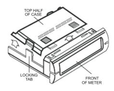
Spread the tabs on each side of the case, using a screwdriver or thumbnail to unlock the top half. Lift the rear of the top half and slide it away from the front of the meter.
