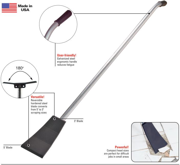
Great for removing tile, wood, laminate, stone, carpet, roofing, and even ice, the Brutus® Reversible Scraper is also excellent for use in tight areas. It features a unique reversible blade which can be easily converted from 5 inches to 3 inches, depending on the worksite needs. The hardened steel blade can be re-sharpened with a grinder or file when necessary. Built with the user in mind, the galvanized steel shaft of the Brutus 62960 has a curved, ergonomic handle that reduces fatigue.
