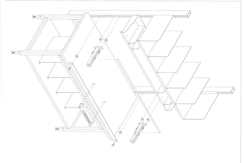
1) MOUNT PAPER SPOOL HOLDER AND ESMR AT DESIRED HEIGHT USING 3/8" X 1" ALLEN CAP SCREWS AND STRUT NUTS
