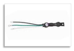
Adapted to SSL outdoor lighting, the Philips SPI surge protection device provides single phase protection for line/neutral, line/ground and neutral/ground in accordance with IEEE C62.41 2002 C High. The SPI small size corresponds to the current design requirements for the new technology luminaires, like a LED light engine in outdoor lighting.
