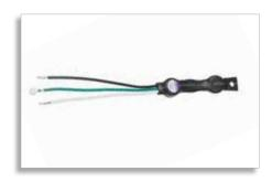
Adapted to SSL outdoor lighting, the Philips SPIHV surge protection device provides all phases protection for line/neutral, line/ground and neutral/ground in accordance with IEEE C62.41.2-2002 C High.The SPIHV small size corresponds to the current design requirements for the new technology luminaires, like a LED light engine in outdoor lighting.
