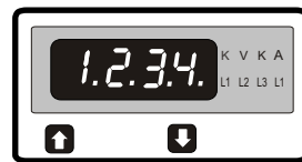
Screen 3 : System Current min. Value Value displayed after "Lo" flashing on Display
