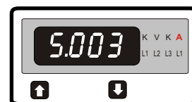
Screen 3 : System Current min. Value Value displayed after "Lo" flashing on Display
