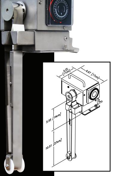
The stainless steel Mighty Mini is a compact belt skimmer designed for parts washers and machine tool coolant sumps. With its large discharge trough and small operating space, the Mighty Mini fits almost anywhere. The stainless steel construction resists rust and corrosion in harsh environments. It is lightweight and requires minimal assembly. With its durable stainless steel construction, it is built to give long lasting performance. The removable trough makes cleanup fast and easy.
