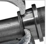
Tapered roller bearing on shaft
