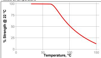
Cured for 5 days @ 22 °C Lap Shear Strength, ISO 4587: Steel
