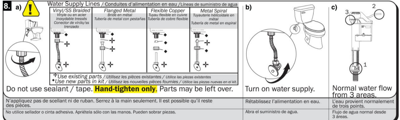
**Do not use sealant / tape. Hand-tighten only.** Parts may be left over.
