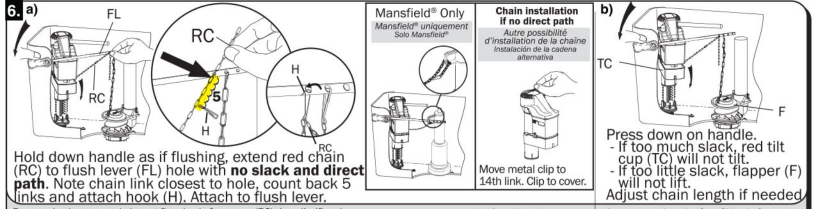
**Hold down handle as if flushing, extend red chain (RC) to flush lever (FL) hole with no slack and direct path.** Note chain link closest to hole, count back 5 links and attach hook (H). Attach to flush lever.
