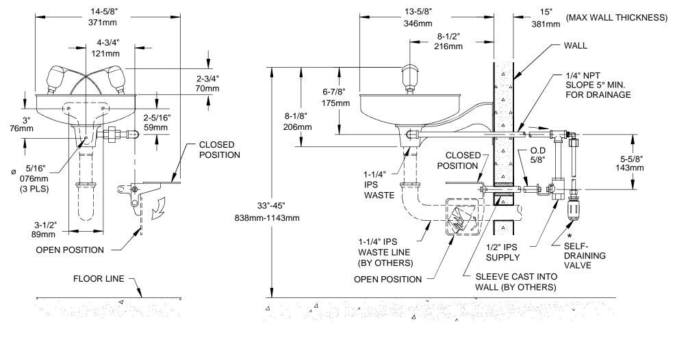
\* VALVE IS SELF-DRAINING, THUS PERMITS STANDING WATER TO DRAIN AFTER EACH USE PREVENTING FREEZE-UPS. PROPER PROVISIONS MUST BE MADE FOR DRAINAGE.
