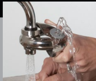
Rotating the front of the eyePOD one-half turn (in either direction) brings the eyewash spouts to the top and automatically resets the unit to operate as an eyewash.
