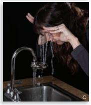
With logo facing upward, faucet functions normally (a). Rotating the front one-half turn (in either direction) brings the eyewash spouts to the top (b) and the unit operates as an eyewash (c).
