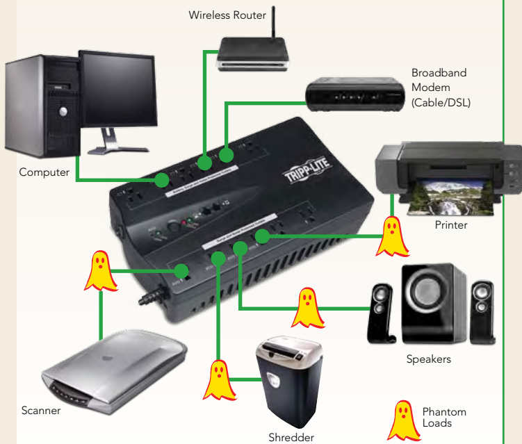
Green Outlet technology cuts power to designated energy-saving outlets when your computer shuts down or enters standby mode, preventing idle devices connected to those outlets from wasting energy. Other outlets stay on to support devices that operate continuously, such as routers and broadband modems.
