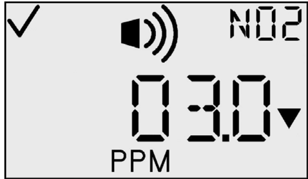
Low Alarm Setpoint Screen
