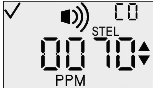
STEL Alarm Setpoint Setup
