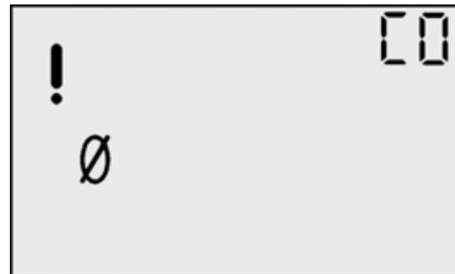
Zeroing Failed Screen
