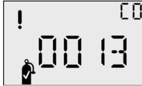
Cal Failed (!) Screen
