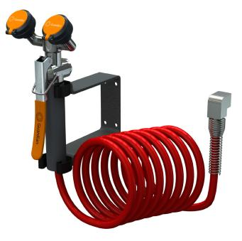
Application: Dual purpose eyewash/drench hose for wall mounting. Unit meets the provisions of ANSI Z358.1-2009 as both an eyewash and a drench hose. Unit may be left in the mounting bracket for use as a fixed eyewash, leaving user's hands free. Alternatively, unit may be removed for use as a drench hose to rinse any part of user's eyes, face or body.
