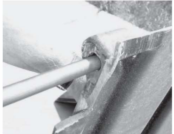
Insert pin through all lid hinge bosses.
