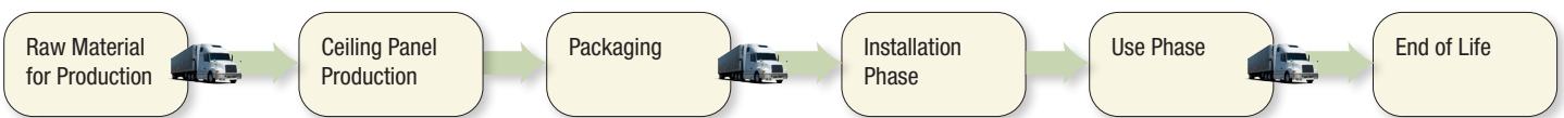
Figure 5. Life cycle phases included for the mineral fiber ceiling panels in study:
