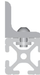
Slide pre-loaded part into T-slot
