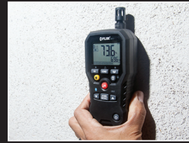
Capture moisture readings up to 0.75" below surfaces
