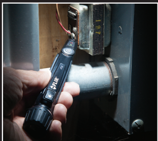
High sensitivity mode is useful for working on low-voltage systems
