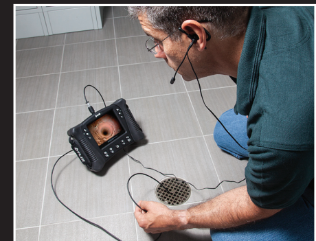
The included headset allows for voice annotations to clarify inspection findings
