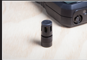
Temperature/humidity sensor is field replaceable
