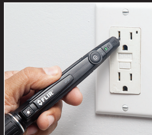
Low-profile tip helps when working with safety outlets.
