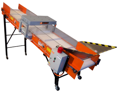
All-metal detectors for even nonferrous metals use transmitter coils (here positioned above the conveyor) and receiver coils to sense a change in the emitted magnetic field caused by metal passing between the coils.
