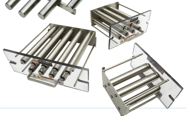
Grate magnets allow dry materials to cascade between magnetic tubes in either a single layer or multiple staggered layers.
