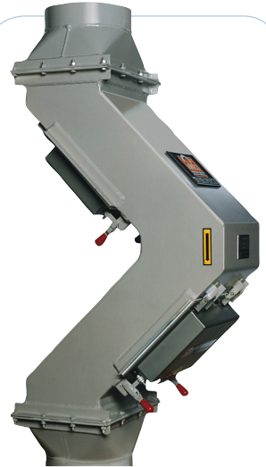
Hump magnets are similar to round pipe separators but use two plate magnets in a dogleg design to increase the chance of ferrous contamination contacting the magnet.
