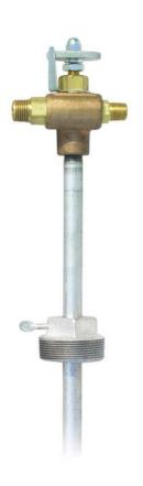
The EconoMixer<sup>™</sup> is designed for speed, accuracy, and cost savings. Simply insert the unit into a 15 – 55 gallon drum of coolant concentrate and connect a water line to the unit. The adjustable needle valve/dial permits any ratio required for instant uniform concentrations. All brass and metal construction. It is equipped with a 2" sliding bung adapter for various height drums. The unit requires 25 pounds of water pressure to operate.
