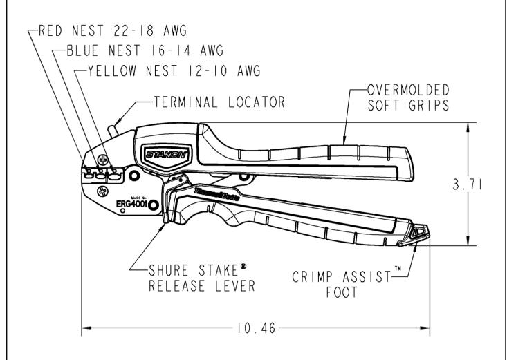
CAUTION: HANDLES NON-INSULATING, DO NOT CRIMP ENERGIZED WIRES
