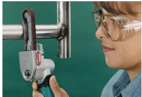
Clean and finish using non-woven nylon belts.
