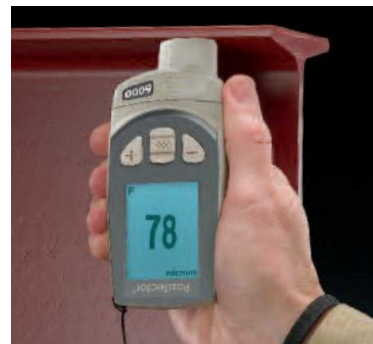
Flip Display enables right-side-up viewing
